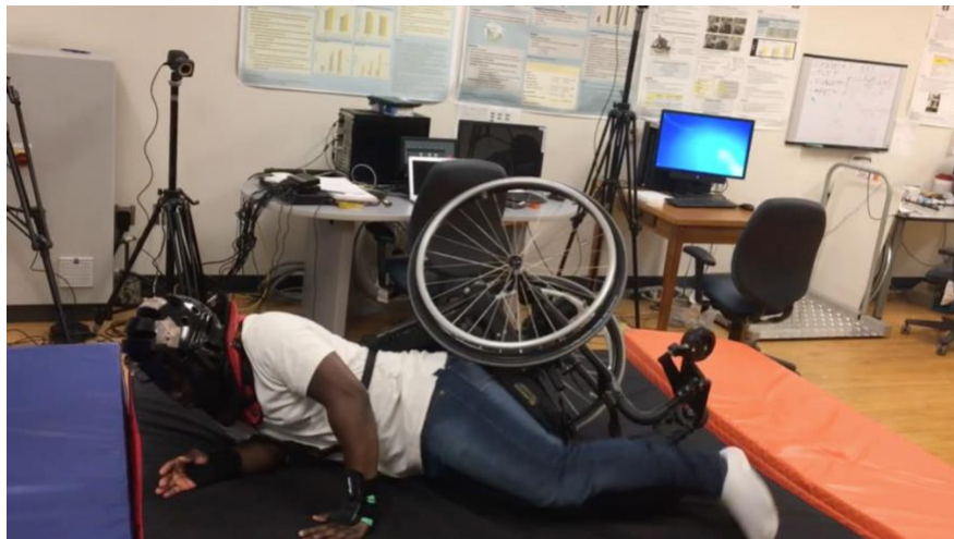
A student does a controlled, forward fall from a wheelchair in the laboratory setting to measure acceleration patterns of different types of falls among wheelchair users.
